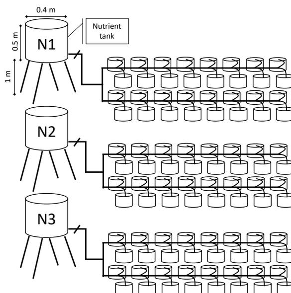
Fig. 1: Layout of experimental design for hydroponic curly endive, with drip systems of three different nutrient concentrations, N1, N2 and N3 are nutrient tanks.
